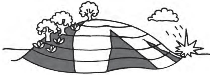
Figure 1.19 Contour lines drawn on a hill to show the areas that are level
