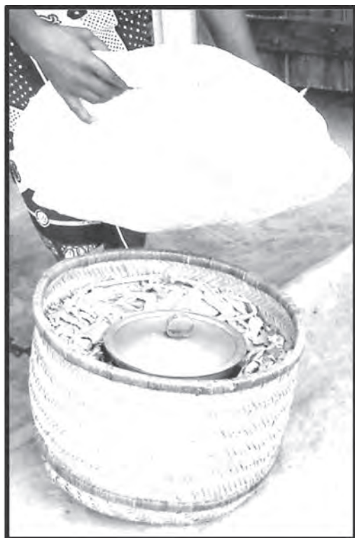
Figure 3.21 Basket cooker with insulated cover
